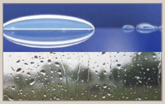
Water beads are more pronounced on the rough surface of ordinary glass, causing more spots and requiring more cleaning.
